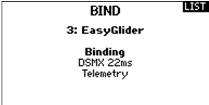
Figure 5: Binding was successful: Receiver and Telemetry detected
