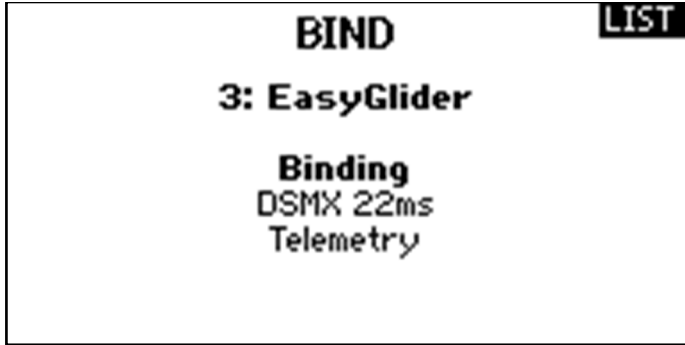
Figure 5: Binding was successful: Receiver and Telemetry detected
